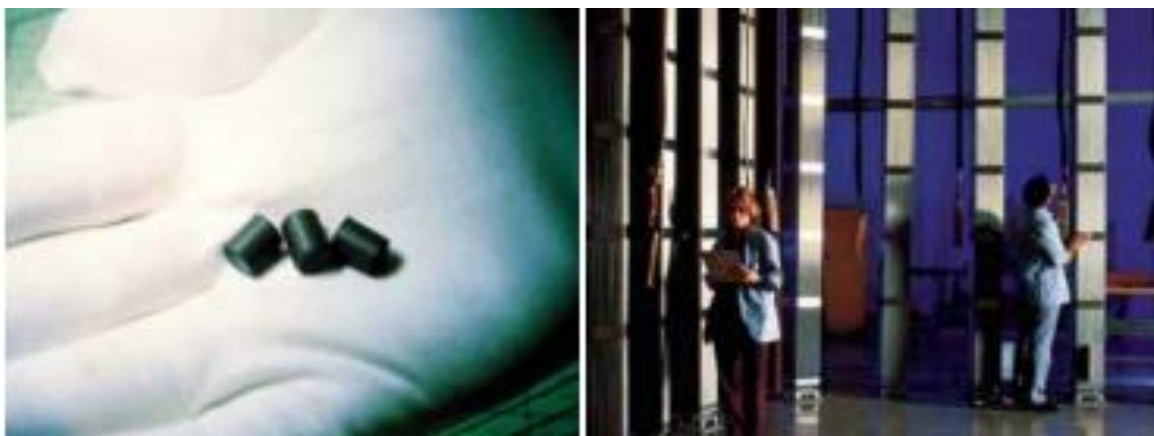
Figure 17-2. (a) Fuel pellets containing enriched uranium-235. Each pellet contains the energy equivalent of 1 ton of coal. (b) Fuel pellets are encased into narrow rods that are bundled together and lowered into the reactor core.
